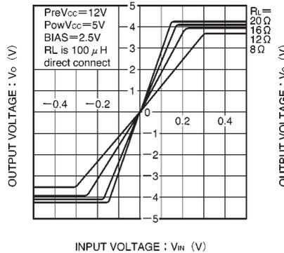
Fig. 12 Driver I/O characteristics (focus and tracking)
